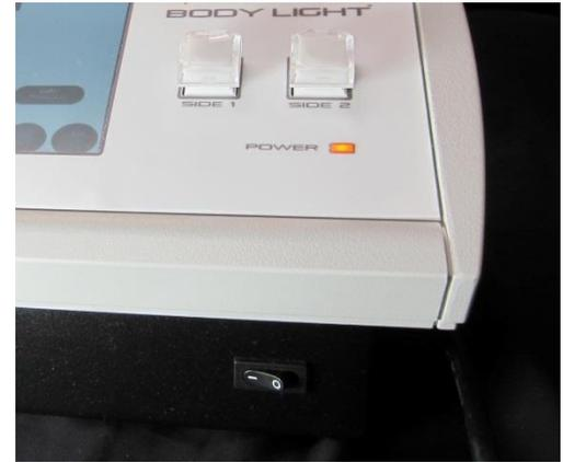
Figure 2 Body Light Power Switch
